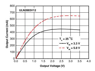
Output Current vs. Output Voltage
