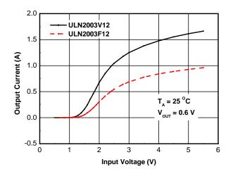
Output Current vs. Output Voltage
