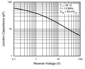
Fig. 5 - Typical Junction Capacitance
