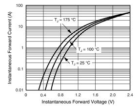
Fig. 3 - Typical Instantaneous Forward Characteristics
