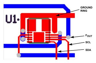
FIGURE 22. SUGGESTED LAYOUT FOR ISL12020M
