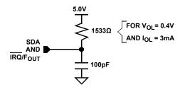
FIGURE 2. STANDARD OUTPUT LOAD FOR TESTING THE DEVICE WITH  $\mbox{V}_{\mbox{DD}} = 5.0\mbox{V}$
