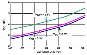
FIGURE 5. I<sub>DD1</sub> vs TEMPERATURE
