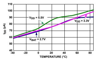
FIGURE 11. I<sub>DD</sub> with TSE = 1 vs TEMPERATURE
