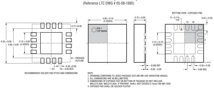
**UF Package** 16-Lead Plastic QFN  $(4mm \times 4mm)$
