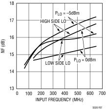
Figure 7. SSB Noise Figure vs Tuned IF Input Frequency
