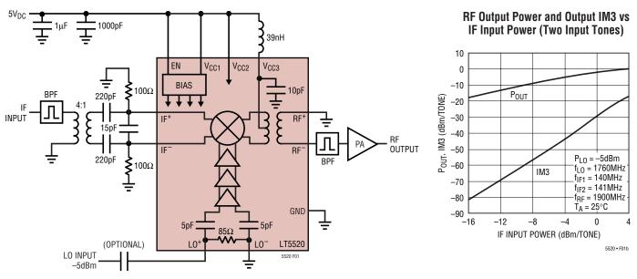
Figure 1. Frequency Conversion in Wireless Infrastructure Transmitter
