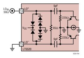
Figure 4. LO Input Circuit
