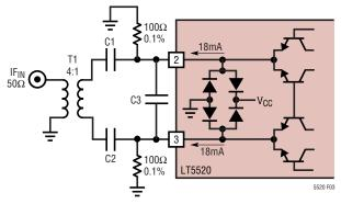
Figure 3. IF Input with External Matching
