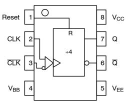
Figure 1. Logic Diagram and Pinout Assignment
