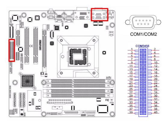
AIMB-581 supports six serial ports. COM1, COM2, COM4-6 supports RS-232. COM3 supports RS-232/422/485(with 5V/12V power). JSETCOM3 is used to select the RS-232/422/485 mode for COM3.
