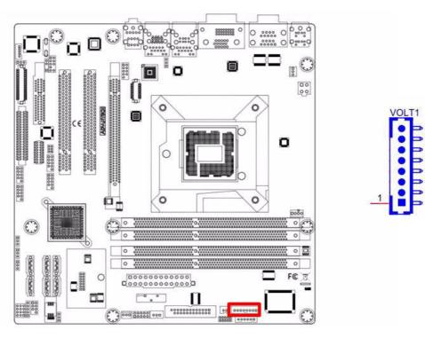
VOLT1 connects to the alarm board of Advantech chassis. These alarm boards give warnings if a power supply or fan fails, if the chassis overheats.
