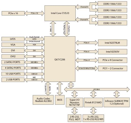
Figure 1.3 AIMB-581 Board Diagram
