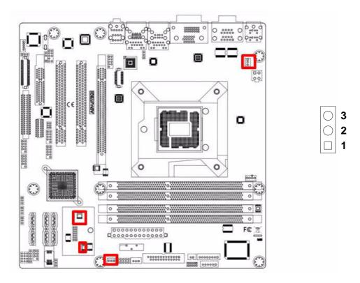
If a fan is used, this connector supports cooling fans of 500 mA (6 W) or less.
