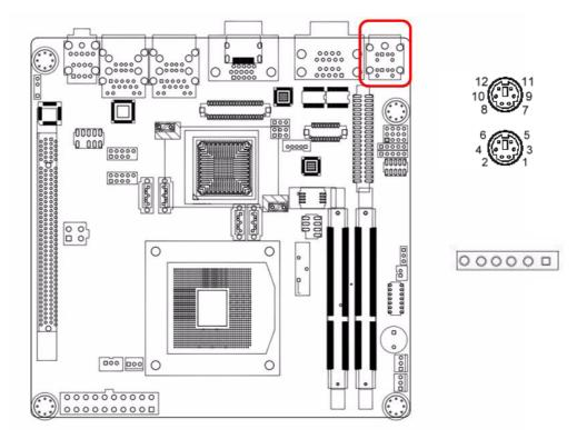
Two 6-pin mini-DIN connectors (KBMS1) on the motherboard provide connection to a PS/2 keyboard and a PS/2 mouse, respectively. KBMS2 is to support the 2nd PS/2 keyboard and PS/2 mouse by a cable P/N 1700018699.
