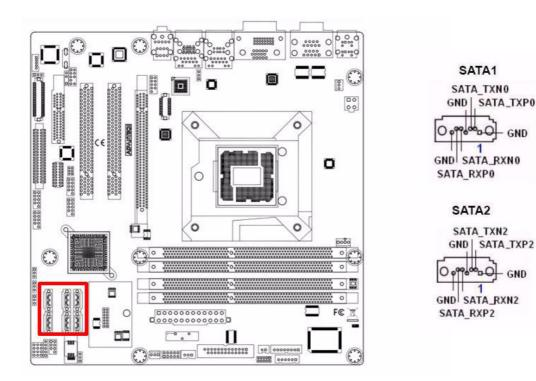
AIMB-581 features a high performance Serial ATA interface (up to 300 MB/s) and Serial ATA III interface (up to 600 MB/s) which eases hard drive cabling with thin, space-saving cables.
