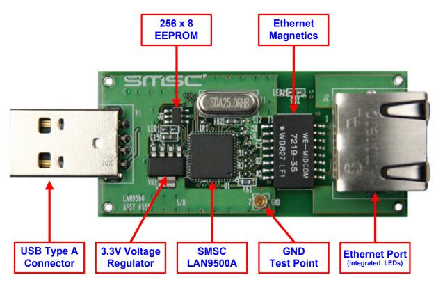
Figure 2.1 EVB-LAN9500A-LC Top View
