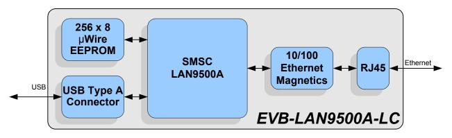
Figure 1.1 EVB-LAN9500A-LC Block Diagram
