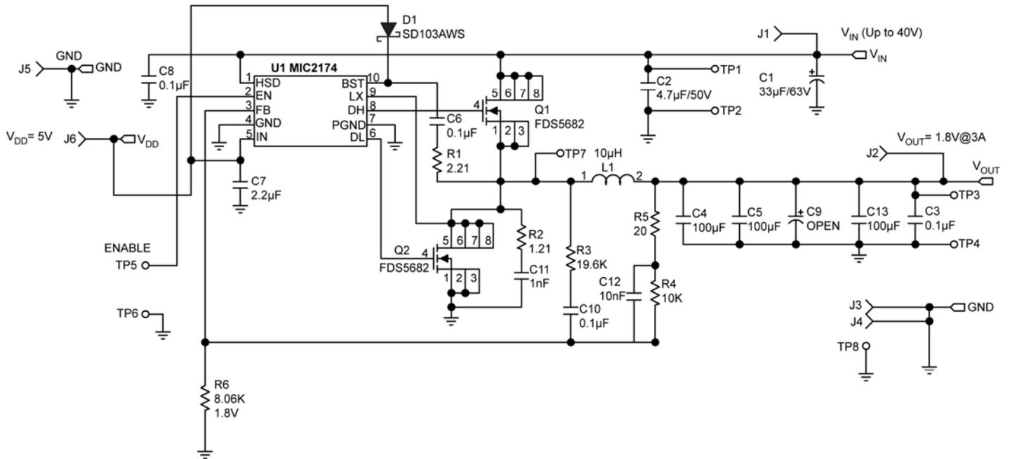
Figure 10. Schematic of MIC2174/MIC2174C Evaluation Board
