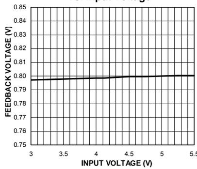
Feedback Voltage vs. HSD Voltage
