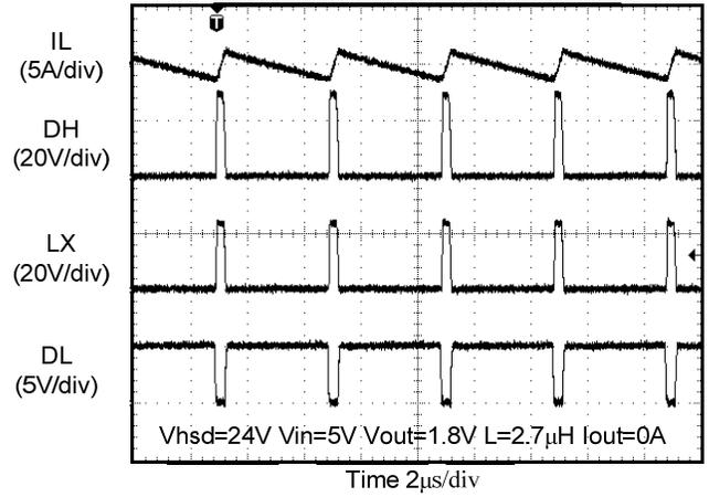
**Switching Waveform (Heavy Load)**
