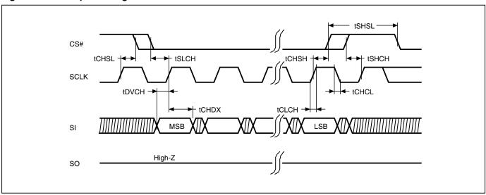
Figure 6. Output Timing
