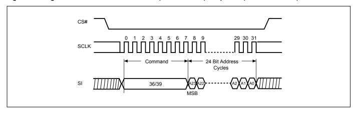
Figure 38. Read Block Protection Lock Status (RDBLOCK) Sequence (Command 3C)
