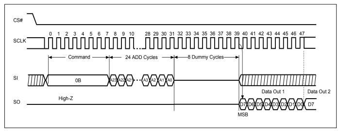
Figure 17. Fast DT Read (FASTDTRD) Sequence (Command 0D)
