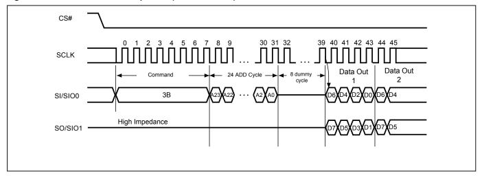
Figure 25. Quad Read Mode Sequence (Command 6B)
