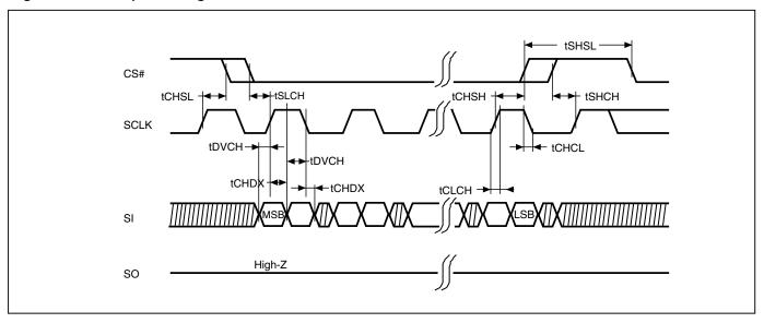
Figure 8. Serial Output Timing for Double Transfer Rate Mode
