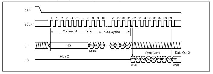
Figure 16. Read at Higher Speed (FAST\_READ) Sequence (Command 0B)
