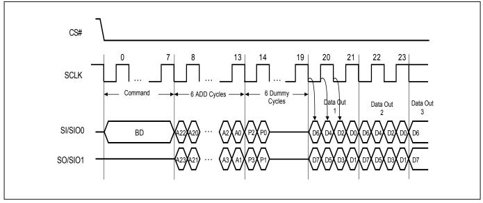
1. SI/SIO0 or SO/SIO1 should be kept "0h" or "Fh" in the first two dummy cycles. In other words, P2=P0 or P3=P1 is necessary.
