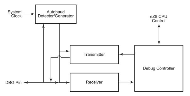
Figure 41. On-Chip Debugger Block Diagram
