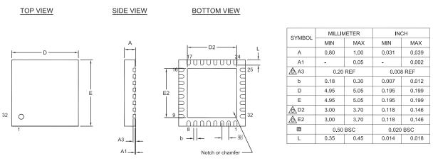
1. CONTROLLING DIMENSIONS : mm 2. MAX. COPLANARITY : 0.08 mm 0.003"
