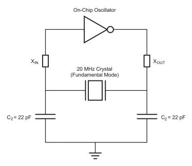
Figure 40. Recommended 20MHz Crystal Oscillator Configuration
