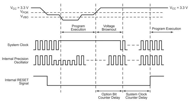
Figure 4. Voltage Brown-Out Reset Operation
