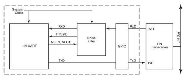
Figure 17. Noise Filter System Block Diagram
