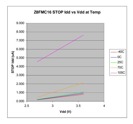
Figure 47. STOP Mode Current Consumption as a Function of Temperature with V<sub>DD</sub> as a Parameter, All Peripherals Disabled
