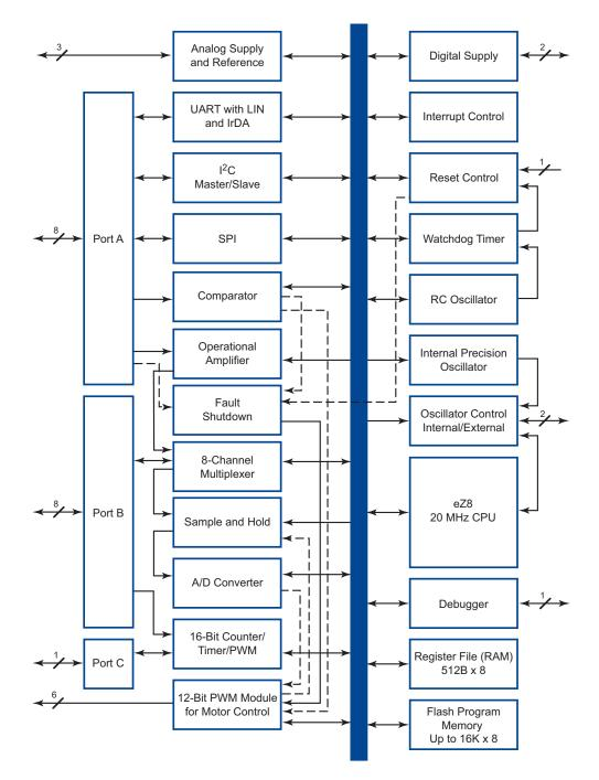
Figure 1. Z8FMC16100 Series MCU MCU Block Diagram
