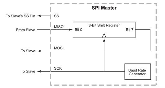
Figure 22. SPI Configured as a Master in a Single Master, Single Slave System
