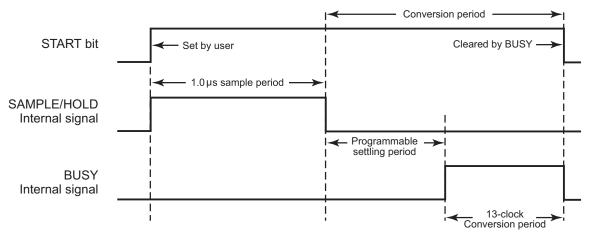
Figure 37. ADC Timing Diagram
