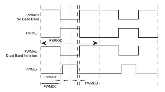
Figure 9. Center-Aligned PWM Output
