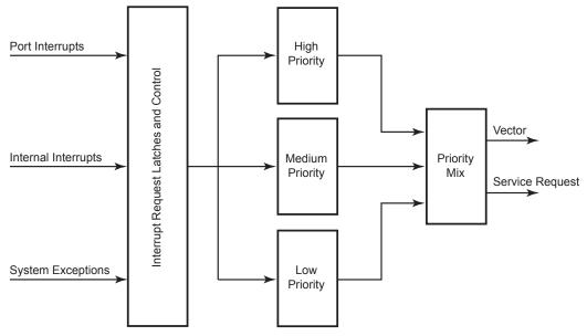
Figure 6. Interrupt Controller Block Diagram
