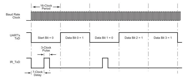
Figure 20. Infrared Data Transmission
