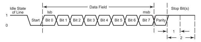
Figure 13. LIN-UART Asynchronous Data Format with Parity
