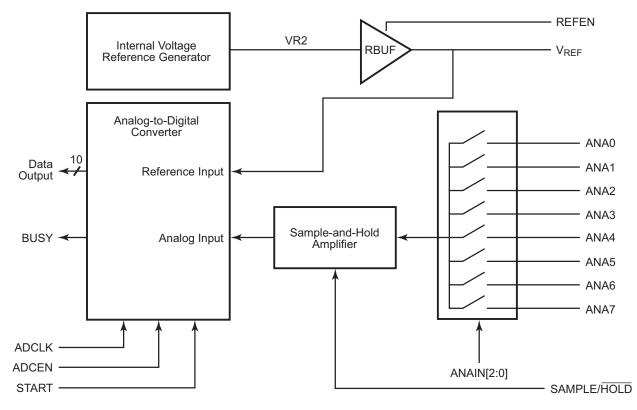
Figure 36. Analog-to-Digital Converter Block Diagram
