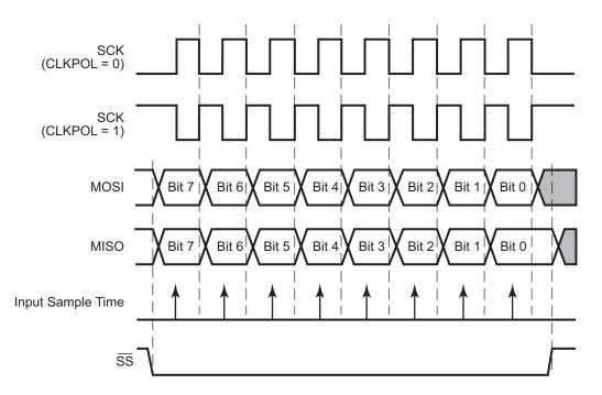
Figure 25. SPI Timing When Phase is 0
