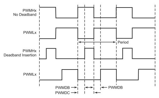
Figure 8. Edge-Aligned PWM Output
