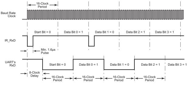
Figure 21. Infrared Data Reception
