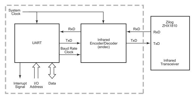
Figure 19. Infrared Data Communication System Block Diagram
