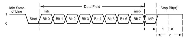
Figure 15. LIN-UART Asynchronous MULTIPROCESSOR Mode Data Format
