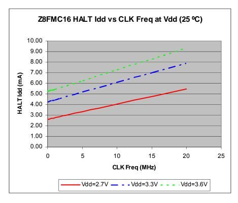
Figure 46. HALT Mode Current Consumption as a Function of Clock Frequency with V<sub>DD</sub> as a Parameter at 25°C
