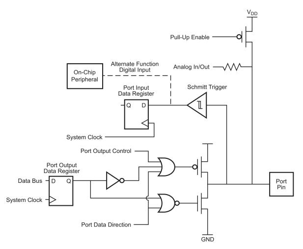
Figure 5. GPIO Port Pin Block Diagram
