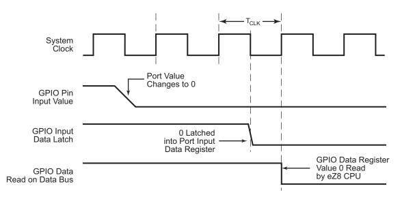
Figure 48. Port Input Sample Timing
