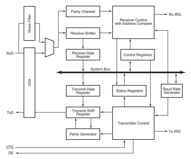
Figure 11. LIN-UART Block Diagram
