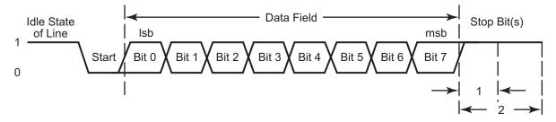
Figure 12. LIN-UART Asynchronous Data Format without Parity
