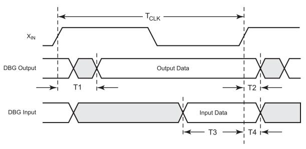
Figure 50. On-Chip Debugger Timing
