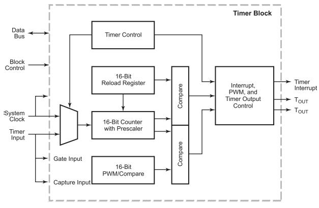
Figure 10. Timer Block Diagram
