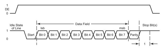
Figure 14. LIN-UART Driver Enable Signal Timing (shown with 1 Stop Bit and Parity)
