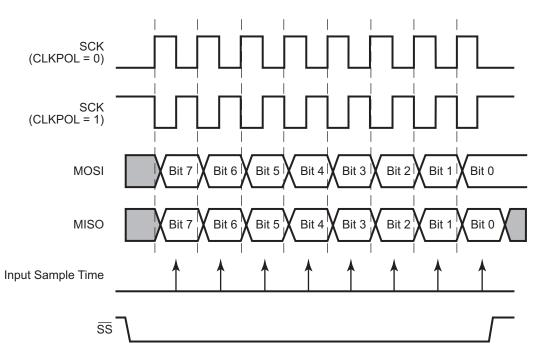
Figure 26. SPI Timing When Phase is 1
