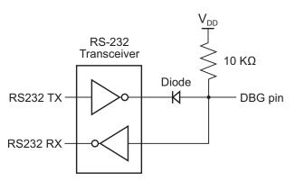
Figure 42. Interfacing the On-Chip Debugger's DBG Pin with an RS-232 Interface, #1 of 2
