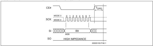
FIGURE 5-14: RELEASE FROM DEEP POWER-DOWN SEQUENCE
