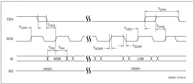
FIGURE 6-4: SERIAL INPUT TIMING DIAGRAM
