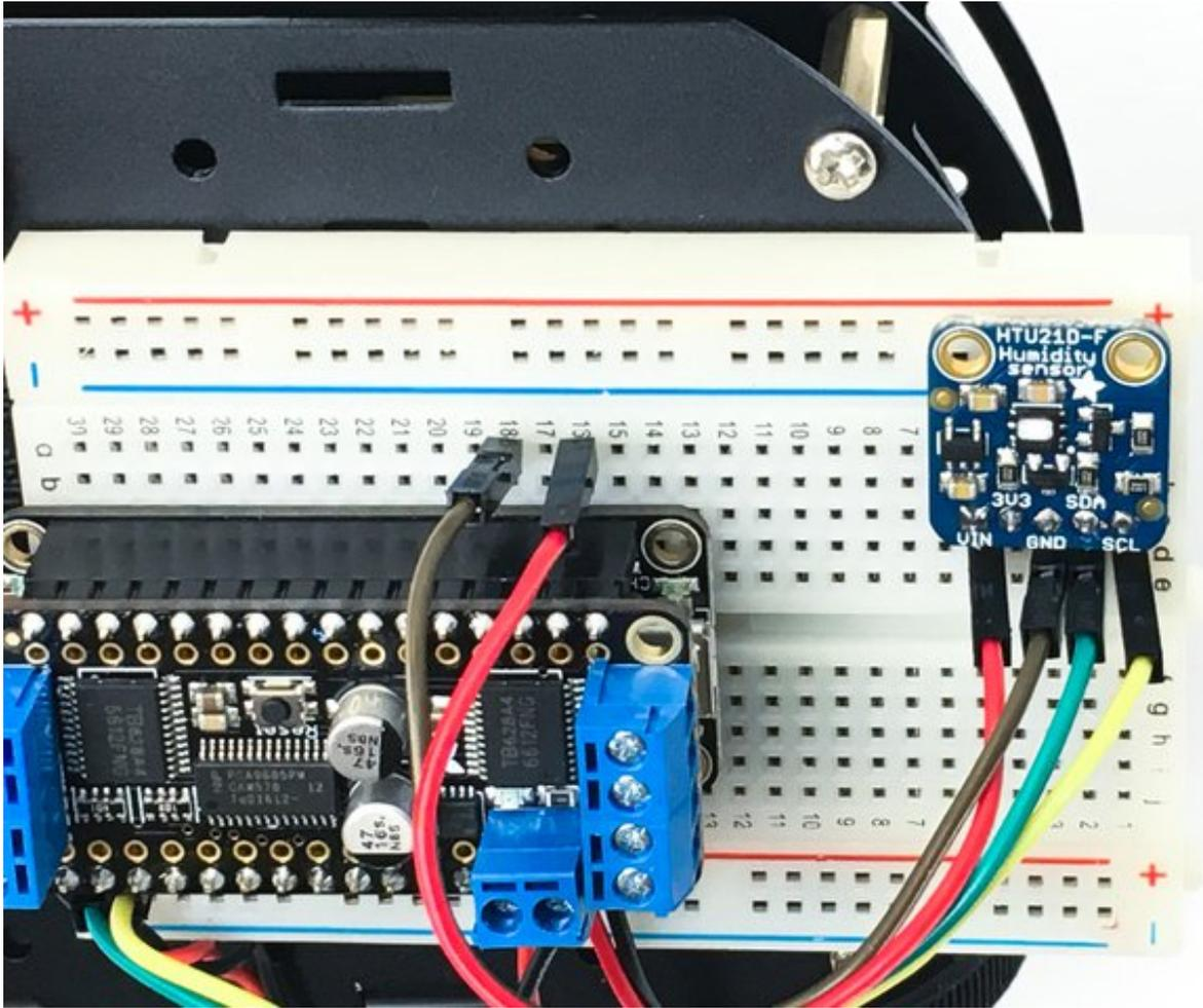
The HTU21D-F has a default I2C address of 0x40 and cannot be changed!
