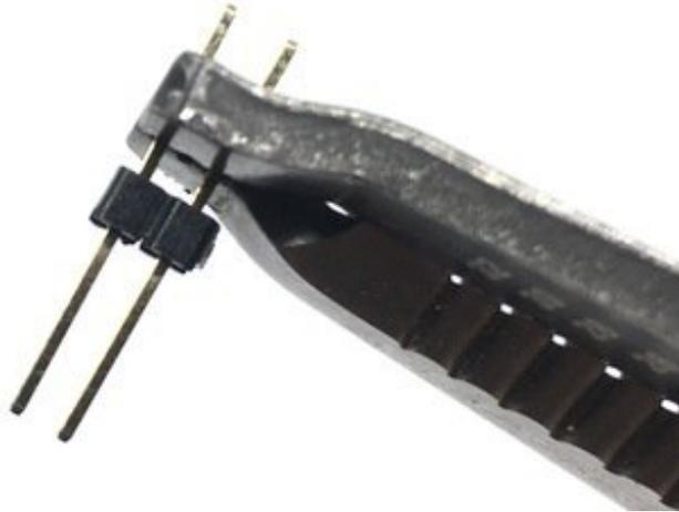
For this next step, a pair of pliers is handy. First, grab the 6 header pins all attached together and break them into 3 sets of 2 header pins. Then, grab them in the pliers like shown here, and then slightly bend them so they look like the next picture.
