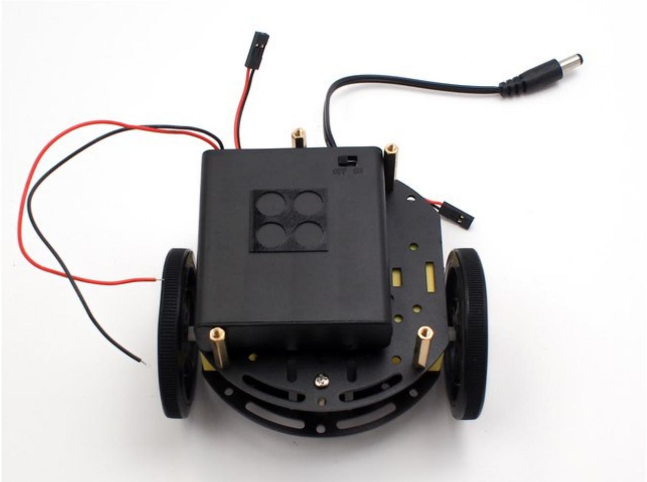
Notice the battery box is lined up on the left side of the middle chassis plate. It should be just in-between the upper left stand-off and the lower left stand-off (not touching either). This will make sure the on-off switch lines up just right in the hole of the top plate. Go ahead and install the top plate now as shown here.
