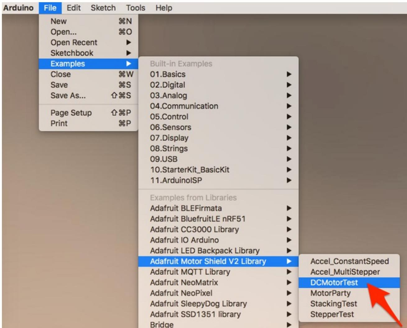
Take a look through this example sketch. Before you upload the code and run it on your robot, you need to make a change or two. First off, you will need to change what port the motors are connected to. Let's start by just trying one of the motors. If you remember when we assembled the robot, we connected the motors to the back of the motor shield, in ports M3, and M4. So, in the top part of the code, go ahead and change out the port from 1, to 3 like this:
