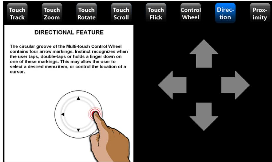
The MTCW's indented outer ring contains four directional arrows (up/down/left/right). Tapping, double-tapping or touch-and-holding a single finger on these markings can be recognized as unique gestures separate from the rest of the touchpad. These gestures are perfect for typical joystick machine control operations.
