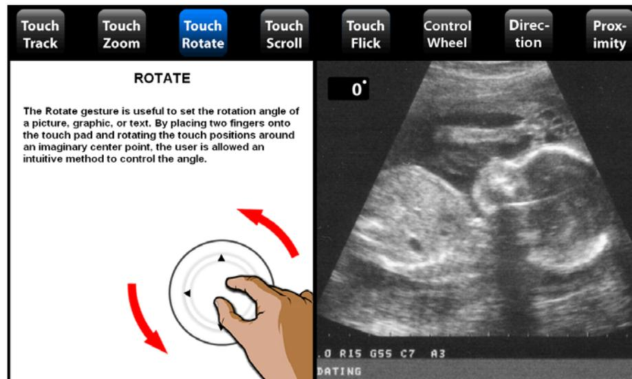
“Touch Rotate” is performed by rotating two touches about each other. It can be useful for rotating pictures, graphics or text on the screen.
