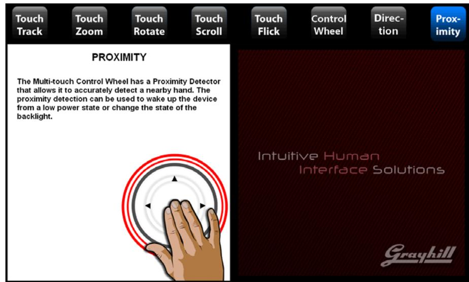
If your product needs to meet green energy requirements, the built in proximity sensor can be a big help. The machine can be placed in a low power state, and when the proximity is sensed, the MTCW can notify the machine that a user is present. For battery powered applications, custom firmware can be written for the MTCW so that even the MTCW itself can be placed in a low power mode - while still monitoring for proximity.
