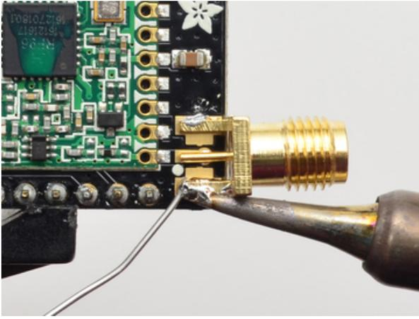
Solder all 5 connections (4 ground/mechanical and 1 signal)
