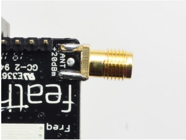
Use plenty of solder to make sure you have a good strong mechanical connection. The duck antennas are long and make great levers, so they could pry apart the solder joints if not soldered well
