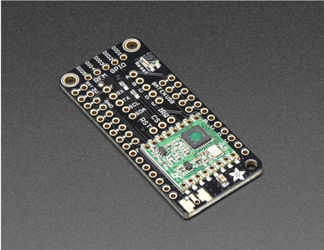
These radio modules come in four variants (two modulation types and two frequencies) The RFM69's are easiest to work with, and are well known and understood. The LoRa radios are exciting, longer-range and more powerful but also more expensive.
