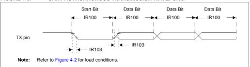
TABLE 4-6: UART ASYNCHRONOUS TRANSMISSION REQUIREMENTS
