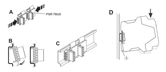
Figure 4 Using the T-BUS DIN rail connector
