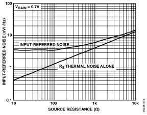
Figure 33. Input-Referred Noise vs. Source Resistance (See Figure 72)
