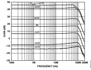
Figure 18. Frequency Response for Various Values of V<sub>GAIN</sub> (See Figure 57)
