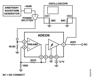
Figure 67. VGA Overdrive Recovery
