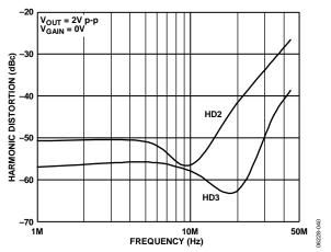
Figure 40. Harmonic Distortion vs. Frequency (See Figure 64)
