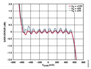
Figure 7. Gain Error vs.  $V_{GAIN}$  for Three Values of Supply Voltage ( $V_s$ ) (See Figure 56)
