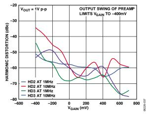
Figure 37. Second and Third Harmonic Distortion vs. V<sub>GAIN</sub> at 1 MHz and 10 MHz (See Figure 64)
