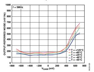
Figure 28. Output-Referred Noise vs. V<sub>GAIN</sub> at Various Temperatures (T) (See Figure 62)
