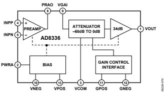
Figure 79. Application Block Diagram
