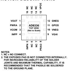
Figure 2. Pin Configuration
