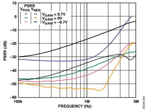
Figure 54. PSRR vs. Frequency for Three Values of V<sub>GAIN</sub> (See Figure 71)
