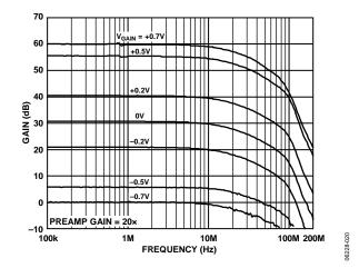
Figure 20. Frequency Response for Various Values of V<sub>GAIN</sub> When the Preamplifier Gain is 20× (See Figure 57)
