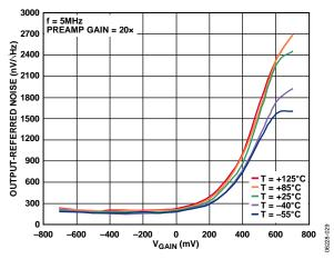
Figure 29. Output-Referred Noise vs. V<sub>GAIN</sub> at Various Temperatures (T) When the Preamplifier Gain is 20× (See Figure 62)
