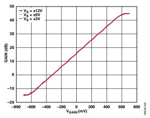
Figure 4. Gain vs.  $V_{GAIN}$  for Three Values of Supply Voltage ( $V_s$ ) (See Figure 56)
