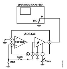
Figure 62. Input-Referred Noise and Output-Referred Noise
