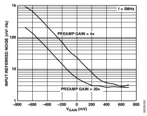
Figure 30. Input-Referred Noise vs.  $V_{GAIN}$  for Preamplifier Gains of 4× and 20× (See Figure 62)
