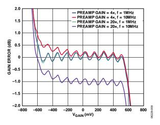
Figure 9. Gain Error vs.  $V_{GAIN}$  at 1 MHz and 10 MHz and for Preamplifier Gains of 4× and 20× (See Figure 56)
