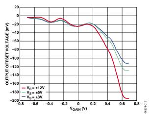
Figure 15. Output Offset Voltage vs. V<sub>GAIN</sub> for Three Values of Supply Voltage (V<sub>s</sub>)
