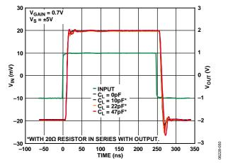
Figure 50. Large-Signal Pulse Response for Various Values of Load Capacitance Using ±5 V Power Supplies (See Figure 65)
