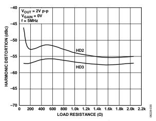
Figure 35. Harmonic Distortion vs. Load Resistance (See Figure 64)
