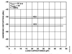
Figure 36. Harmonic Distortion vs. Load Capacitance (See Figure 64)
