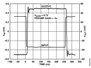
Figure 46. Inverting Gain Small-Signal Pulse Response (See Figure 70)
