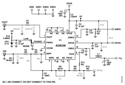
Figure 88. AD8336-EVALZ Schematic Shown as Shipped, Configured for a Noninverting Gain of  $4\times$
