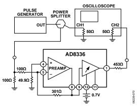
Figure 70. Pulse Response, Inverting Gain
