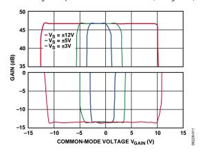
Figure 11. Gain vs. Common-Mode Voltage at VGAIN
