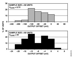
Figure 16. Output Offset Histogram
