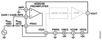
Figure 81. Circuit Configuration for Inverting Gain
