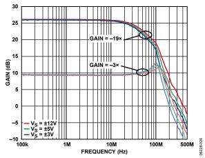
Figure 24. Preamplifier Frequency Response for Three Values of Supply Voltage ( $V_5$ ) When the Inverting Gain Value is  $-3 \times$  or  $-19 \times$  (See Figure 69)
