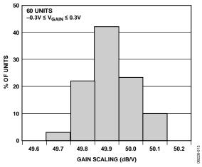
Figure 13. Gain Scaling Factor Histogram
