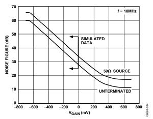
Figure 34. Noise Figure vs. V<sub>GAIN</sub> (See Figure 63)
