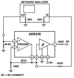
Figure 58. Frequency Response of the Preamplifier
