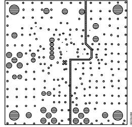
Figure 87. Internal Power Plane Copper
