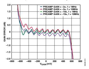
Figure 10. Gain Error vs.  $V_{GAIN}$  at 1 MHz and 10 MHz and for Inverting Preamplifier Gains of  $-3 \times$  and  $-19 \times$  (See Figure 56)
