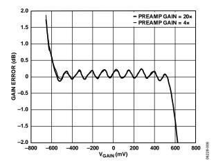
Figure 8. Gain Error vs. V<sub>GAIN</sub> for Preamplifier Gains of 4× and 20× (See Figure 56)
