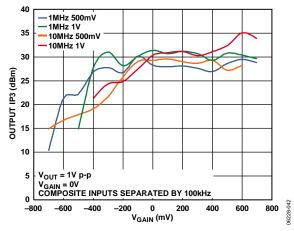
Figure 42. Output-Referred IP3 (OIP3) vs. V<sub>GAIN</sub> at Two Frequencies and Two Input Levels (see Figure 76)
