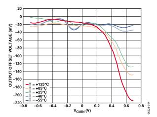
Figure 14. Output Offset Voltage vs. V<sub>GAIN</sub> for Various Values of Temperature (T)
