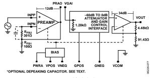
Figure 77. Simplified Block Diagram
