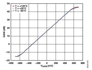
Figure 3. Gain vs. V<sub>GAIN</sub> for Three Values of Temperature (T) (See Figure 56)
