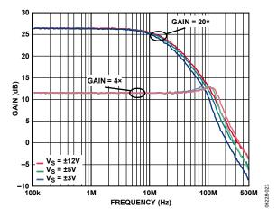
Figure 23. Preamplifier Frequency Response for Three Values of Supply Voltage ( $V_5$ ) When the Preamplifier Gain is  $4 \times$  or  $20 \times$  (See Figure 58)
