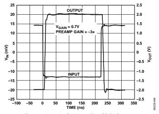
Figure 48. Inverting Gain Large-Signal Pulse Response (See Figure 70)
