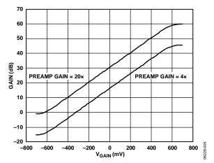
Figure 5. Gain vs.  $V_{\text{GAIN}}$  for Preamplifier Gains of 4× and 20× (See Figure 56)
