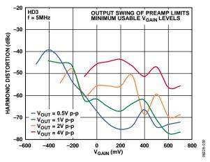
Figure 39. Third Harmonic Distortion vs. V<sub>GAIN</sub> for Four Values of Output Voltage (V<sub>OUT</sub>)
