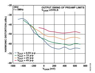
Figure 38. Second Harmonic Distortion vs. V<sub>GAIN</sub> for Four Values of Output Voltage (V<sub>OUT</sub>) (See Figure 64)
