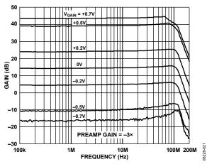
Figure 21. Frequency Response for Various Values of V<sub>GAIN</sub>
