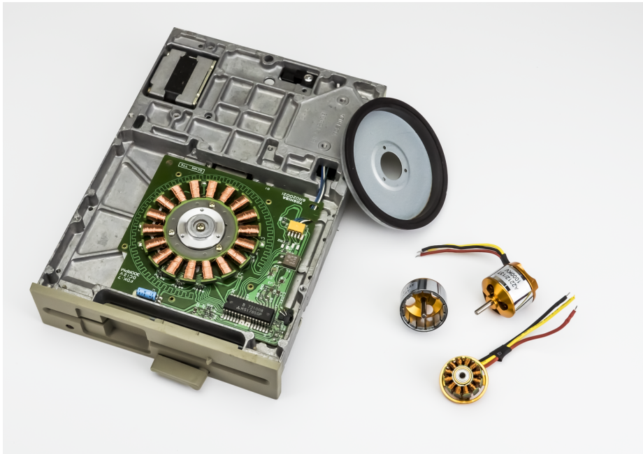
Figure 1-3 Modern drones and old floppy drives use similar brushless motors
