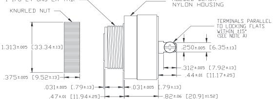
NOTE A: TERMINALS-.032 BRASS TIN PLATED, TAPPED FOR #6-32 SCREW. TWO #6-32 NICKEL PLATED BRASS SCREWS INCLUDED. WILL ACCEPT 1/4" QUICK CONNECT.
