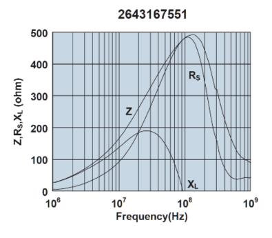
Impedance, reactance, and resistance vs. frequency.
