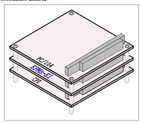
Figure 5. Stack Arrangement Example
