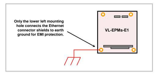
Figure 2. Attaching the VL-EPMs-E1 to Earth Ground
