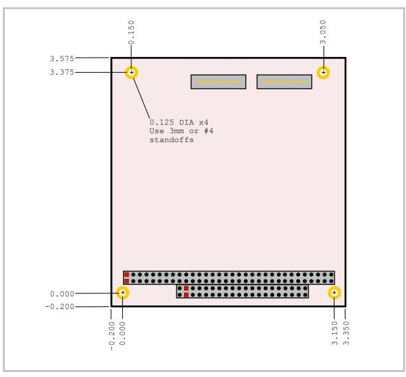
Figure 3. VL-EPMs-E1 Dimensions and Mounting Holes (Not to scale, All dimensions in inches.)
