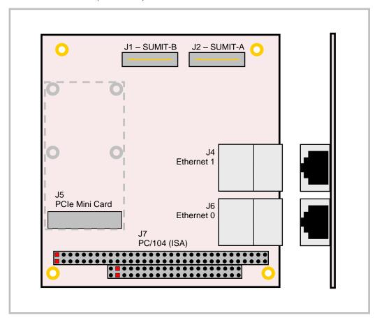
Figure 6. VL-EPMs-E1b Connectors - Top Side
