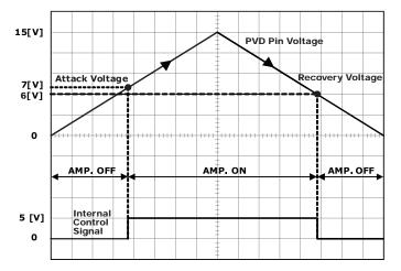
Figure 4.1 Under voltage protection circuit operation
