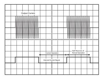
Figure 4.3 Thermal protection circuit operation
