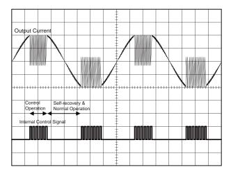
Figure 4.2.1 Graphical representation of overcurrent protection circuit operation
