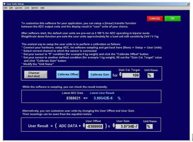
Figure 11. User Units Setup Window
