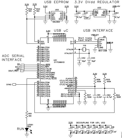
Figure 13. EVAL-AD7194EBZ Schematic, Digital Part
