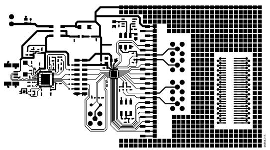
Figure 15. EVAL-AD7194EBZ Component Side View
