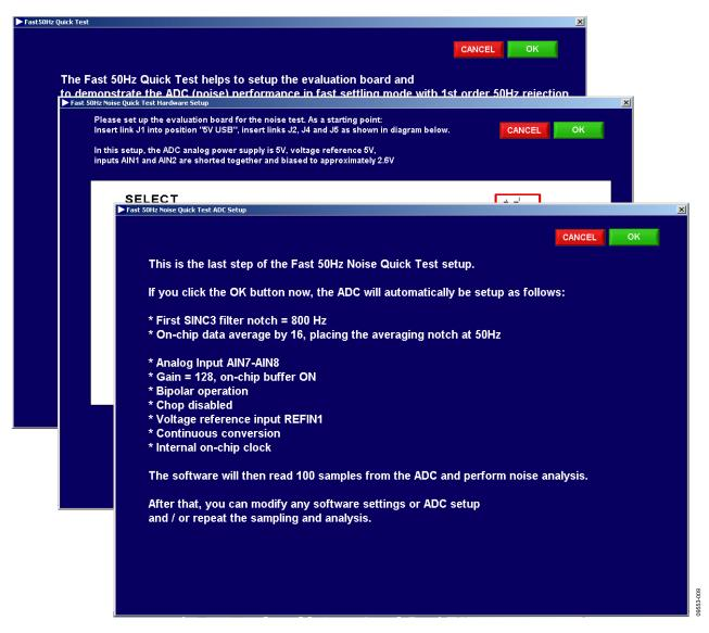
Figure 9. Fast 50 Hz Quick Test
