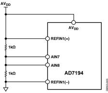
Figure 3. Noise Test Connections
