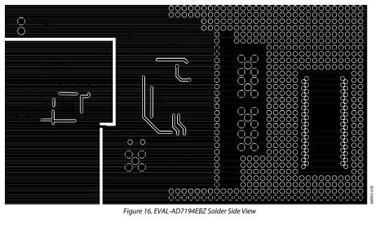
Figure 16. EVAL-AD7194EBZ Solder Side View
