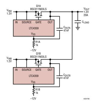
Figure 8. 1.2V Diode-OR
