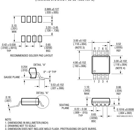
**MS8** Package 8-Lead Plastic MSOP (Reference LTC DWG # 05-08-1660 Rev G)
