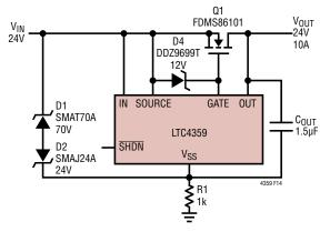
Figure 14. 24V Ideal Diode with Reverse Input Protection
