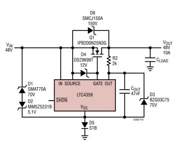
Figure 10. 48V Ideal Diode with Reverse Input Protection
