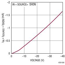
Gate Current vs Forward Voltage Drop
