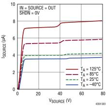
OUT Current vs Forward Voltage Drop
