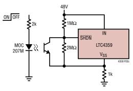
Figure 4c. Opto-Isolator SHDN Control
