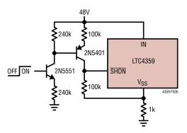
Figure 3b. Transistor SHDN Control
