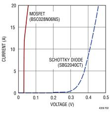
Figure 2. Forward Voltage Drop Comparison Between MOSFET and Schottky Diode
