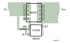
Figure 7b. Layout, MS8/S8 Package
