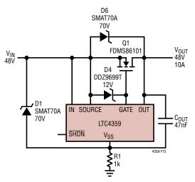
Figure 15. 48V Ideal Diode without Reverse Input Protection
