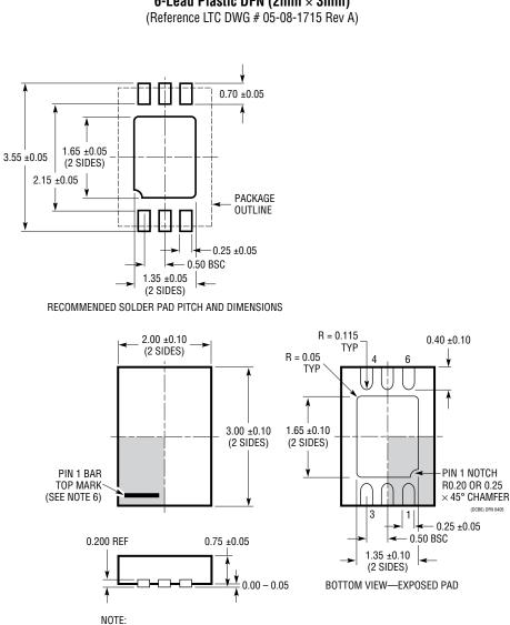
DCB Package 6-Lead Plastic DFN (2mm × 3mm)
