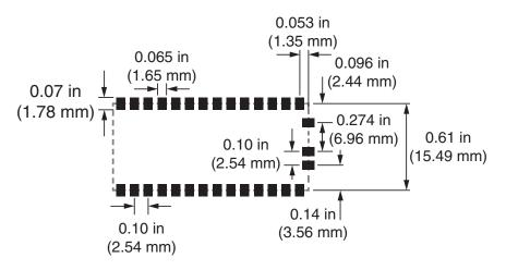
Figure 21: Recommended PCB Layout
