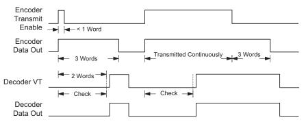
Figure 13: Encoder / Decoder Timing Diagram
