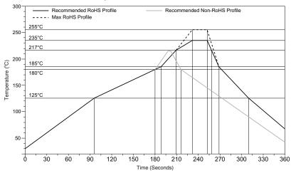
Figure 26: Maximum Reflow Temperature Profile
