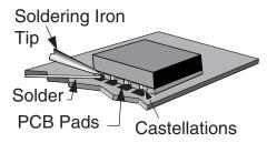
Figure 24: Soldering Technique
