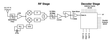
Figure 11: KH3 Series Receiver Block Diagram
