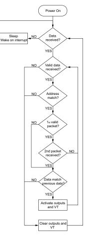
the outputs to briefly cut out when a line is Flowchart toggled.
