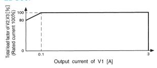
■By V2 load condition, the load factor of V3 is changed as below.
