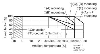
In the hatched area, the specification of Ripple, Ripple Noise is different from other area.
