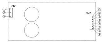
①Frame ground 2AC(N) 3AC(L) **4V1 Output 5V1 Output**
