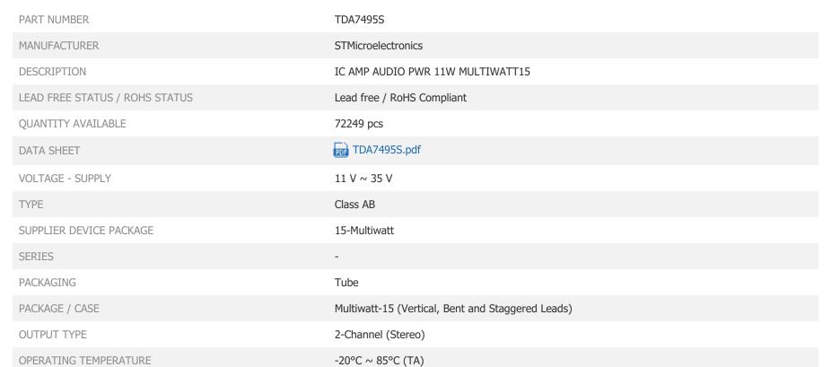
MOUNTING TYPE Through Hole MOISTURE SENSITIVITY LEVEL (MSL) 3 (168 Hours) MAX OUTPUT POWER X CHANNELS @ LOAD 11W x 2 @ 8 Ohm
